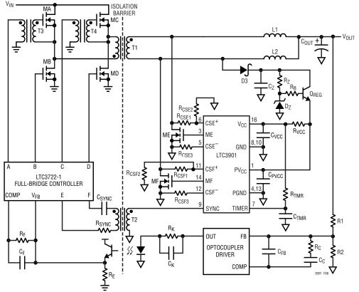
Figure 9. Simplified Isolated Full-Bridge Converter
