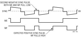
Figure 5. SYNC Double Pulse Operation
