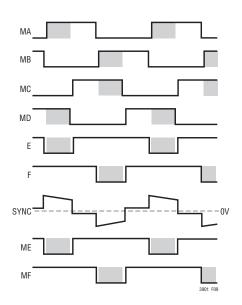
Figure 10. Full-Bridge Converter Switching Waveforms
