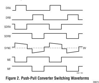
In the second period, SDRA goes high and T2 provides approximately 0V at the LTC3901 SYNC input. This causes the LTC3901's ME output to go high and both MOSFET ME and MF to conduct. This is the free-wheeling period with T1 secondary winding shorted.
