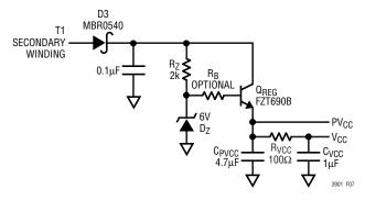
Figure 8. V<sub>CC</sub>/PV<sub>CC</sub> Regulator
